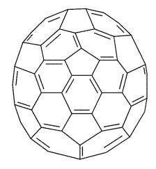
$C_{70}$  Fullerene is the "big brother" of  $C_{60}$ . It has a much stronger absorption of visible light, which is very advantageous in for example (organic) solar cells. Our  $C_{70}$  is very well suitable for organic synthesis purposes. It has a purity of >99% by HPLC, and it is supplied as fine powder and/or crystals which are easy to handle and dissolve.
